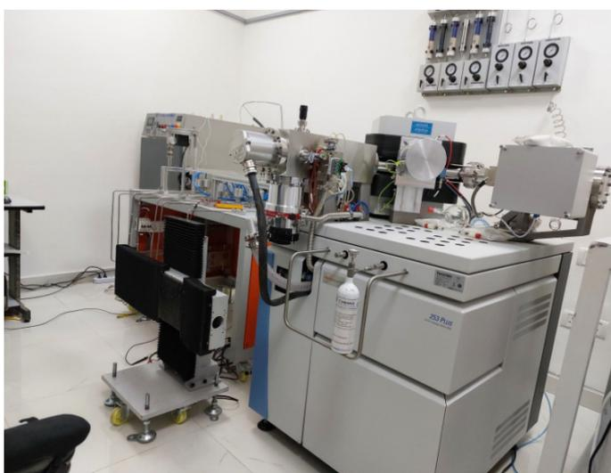
Fig. 2. Thermo Finnigan MAT 253+ mass spectrometer
