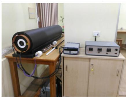
TD-48 Thermal Specimen Demagnetizer
