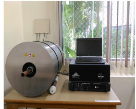
D2000 Alternating Field Demagnetizer
