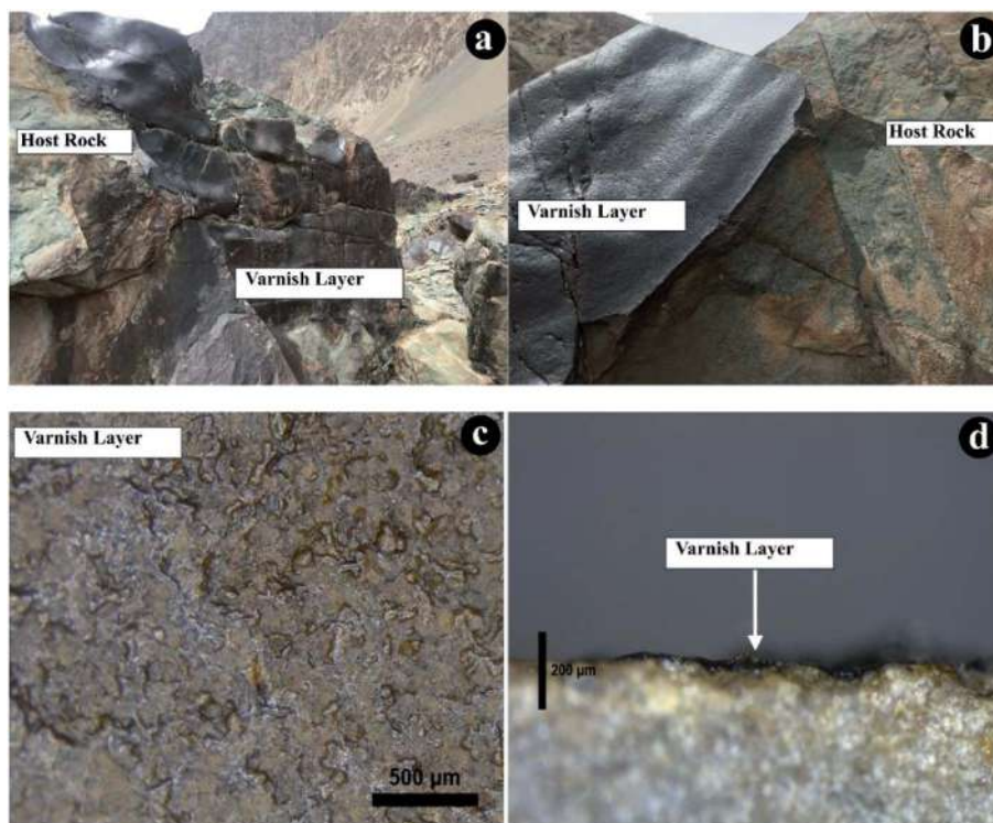
Fig. 1 (a) Synoptic view of varnish coated rock boulders in the field; (b) close-up photograph of the boulder displaying dark rich varnish coated onto the host rock; (c) microscopic image of top varnish layer; (d) cross-sectional view of varnish sample under an optical microscope.
