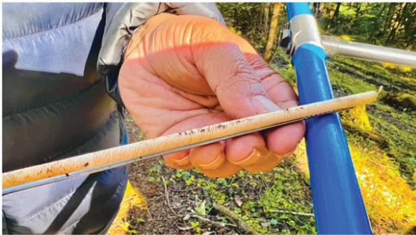
Tree core collection using increment borer
